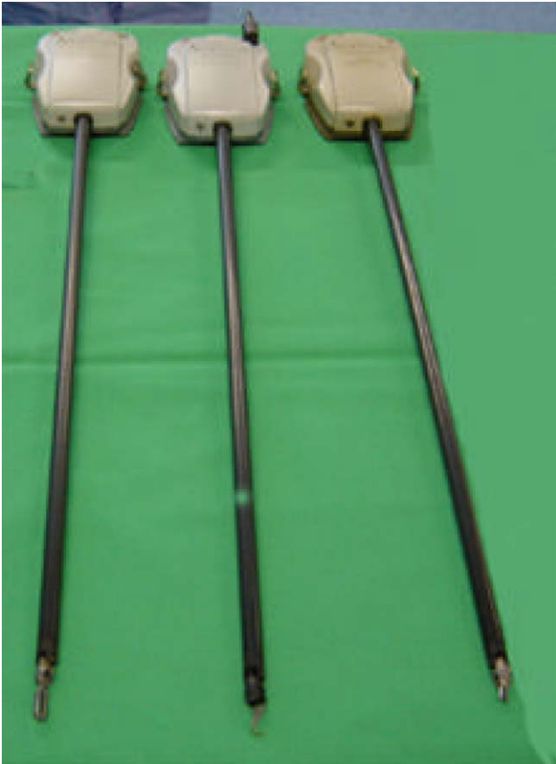
Fig. 2. The Da Vinci robotic system's specific tools (hook, scissors, forceps and needle holder).
